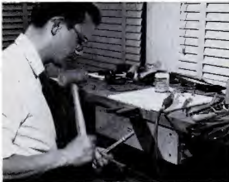
Final shaping of ring is accomplished by slipping it over a mandrel and hammering into a perfect circle before polishing
